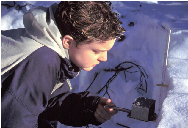
A McGrath student collects a 200 cubic centimeter snow sample using the density sampling box
