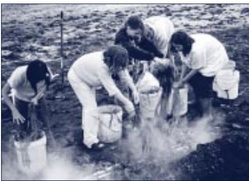
Nasquluk (kelp) was laid on top of the prepared spruce rims which were laid on top of layer of nasquluk, rocks and fire. This combination created the steam necessary to bend the wood for drum rims. Jim Dillard worked with students and adults to make this a highlighted event during both camps.
